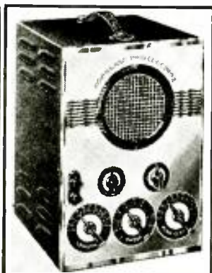
This new oscilloscope, in contrast with more common types, operates on electro-mechanical principles. (1343)
